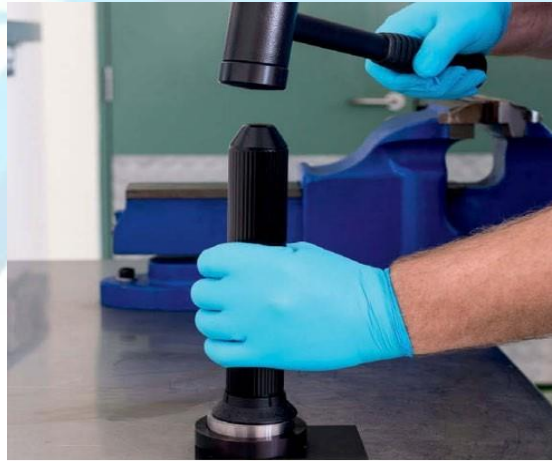
Figure 7: Bearing driving by cold mounting
